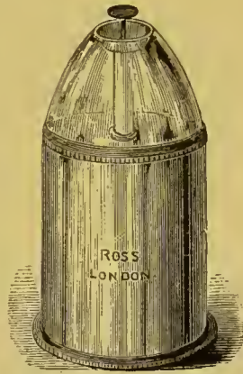
Fig. 144.—Wenham's Parabolic Reflector.
